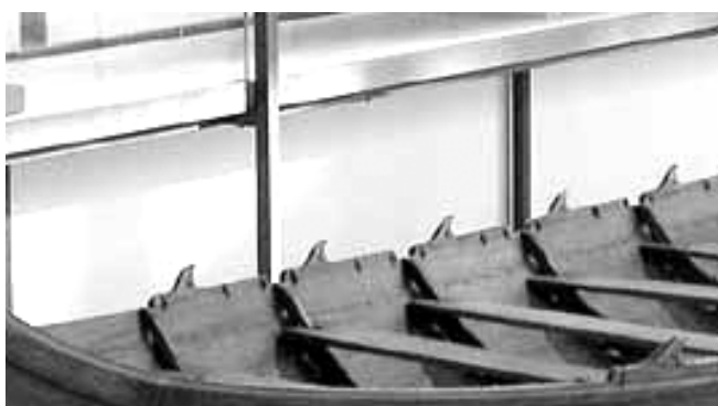
Figure 14: Detail of Kvalsund ship reconstruction... Sheer (top) strake and "crook" tholes.
